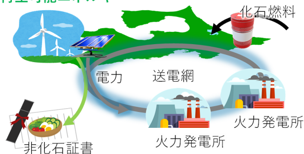
Fig. 1 schematic diagram of connecting renewable energy to the power grids. Electricity value and non-fossil value are separated when connected to the power grids.
