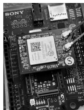
Fig. 3 External antenna connectors and ELTRES add-on board on the Spresense extension board.
