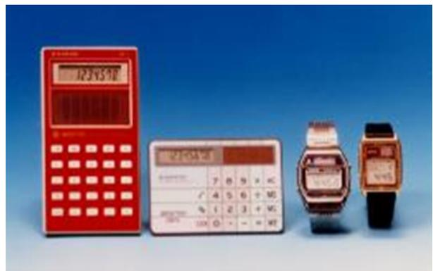
Fig. 3 The world's first solar calculator (left) and solar wristwatch (right) equipped with integrated a-Si solar cells.
