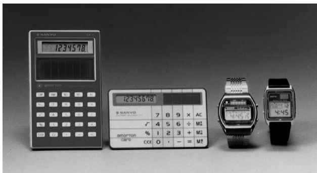
Fig. 1 The world's first solar calculator (left) and solar wristwatch (right) equipped with integrated amorphous silicon solar cells.
