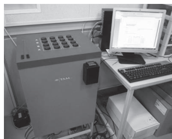
Temperature Range : 5 - 90°C Stability : ±0.02°C
