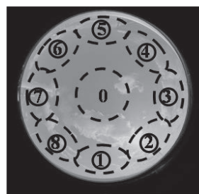
Fig.8 Analysis area of cloud cover by using cloud images 図8 雲画像の遠方雲量推定に用いた解析領域
