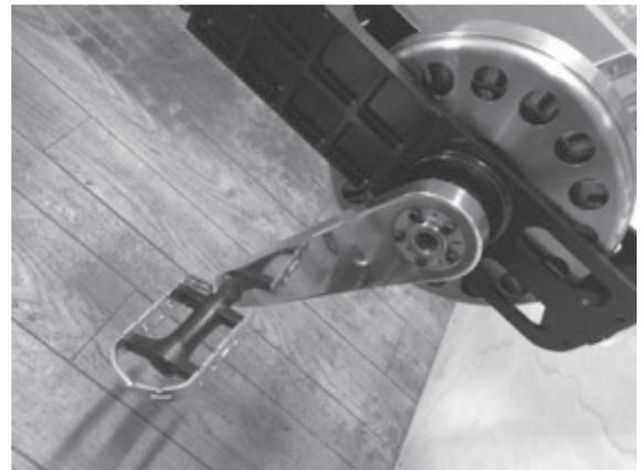
Fig. 11 Direct drive motor and mounter, pedal
