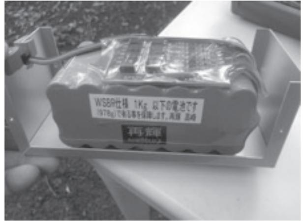
Fig. 5 Li-ion Battery
