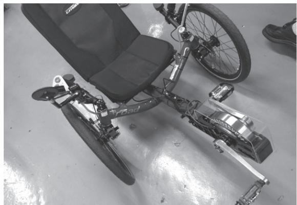
Fig. 13 Direct drive motor with a cover
