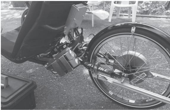
Fig. 14 Driving Motor
