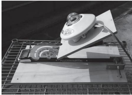
Fig. 4 Pyranometer attached to an inclined surface
