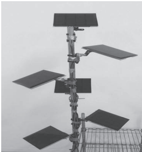
Fig.3: Quasi FPM using the square PV cell.
