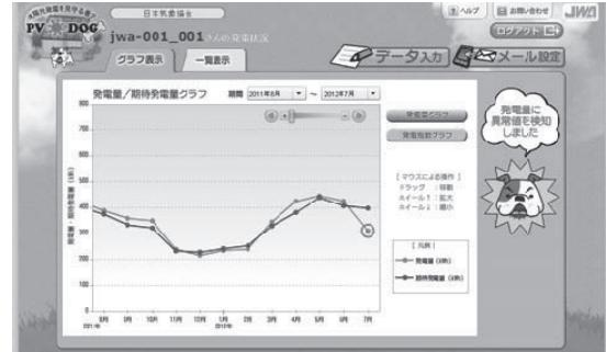
Fig.3 Example of PV-DOG's diagnosis of PV malfunction
