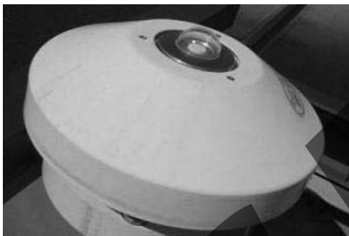
Measurement system: MS-700(350~1050nm)
