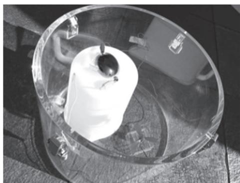
Fig. 14 Operating test of propeller under natural sunlight
