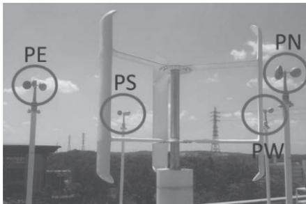
Fig.6 Appearance of anemometer
