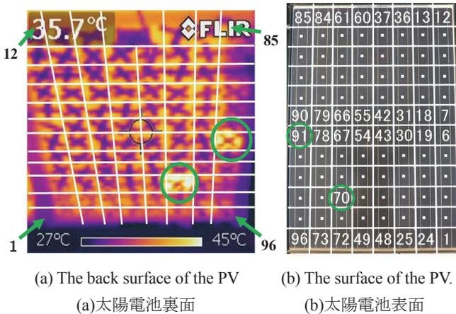
(a) The back surface of the PV (b) The surface of the PV.
