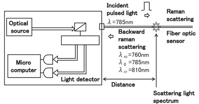
Fig. 3 Composition of the measurement system.
