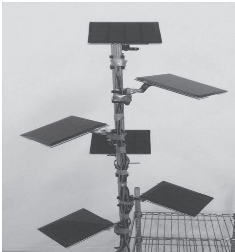
Fig.3: Quasi FPM using the square PV cell.
