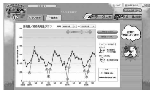
Fig.8 Result of PV-DOG 's diagnosis (NO.49)
