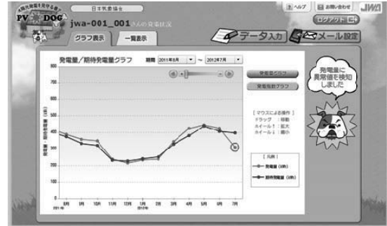
Fig.3 Example of PV-DOG's diagnosis of PV malfunction
